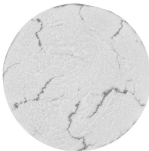
Figure 4 Typical cross-section of a 3.2 mm diameter, glass-fibre-reinforced specimen stressed in torsion at 4 K.
